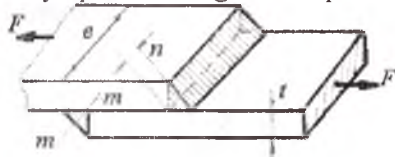
4.13-rasm. Ustma-ust payvandlash.
