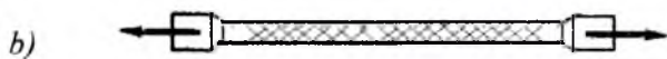
2.12-rasm. Yumshoq po'lotni cho'zilish diagrammasi (a) va (b) namunani oquvchanlik chegaradagi korinishi
