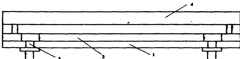
5.3-rasm. Nusxa ko'chiruvchi ramaning vakuumlash sistemasi: 1 – stol, 2 – rezina material; 3 – shtuser; 4 – kvarts shisha.
