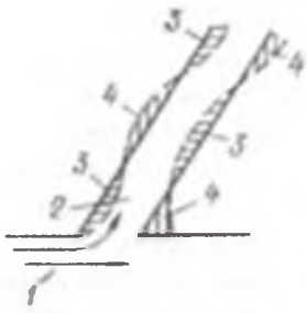
7.33-rasm. Suv olish kallaklarini daryo oqimi yo'nalishi bo'yicha siljishi: 1-daryo, 2-kanal, 3-loyqa to'planish zonasi; 4-yuvilish zonasi
