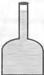
2-rasm. Eng oddiy piknometr.
