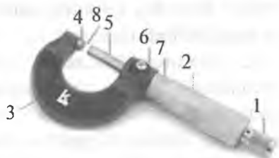
2-rasm. Mikrometrning tuzilishi.
