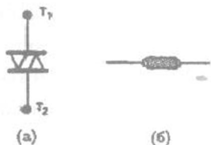
2.54-rasm. Simmetrik diodli tiristor: shartli belgisi (a) va tashqi ko'rinishi (b)
