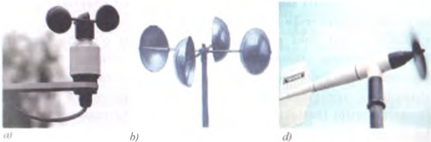
51-rasm. Uch ( a ) va to'rt( b )pallali hamda parrakli ( d ) anemometrlar.
