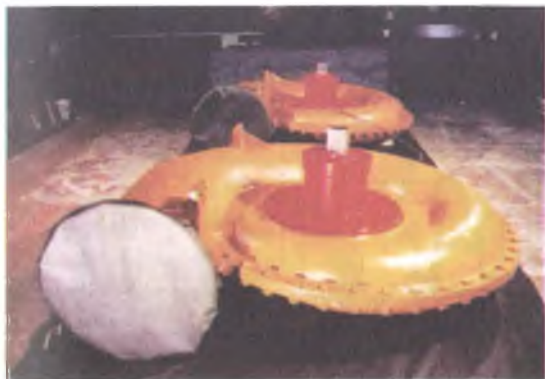
40-rasm. Vertikal (a) va gorizontal (b) o'rnatiladigan radial-o'qiy turbinalar.
