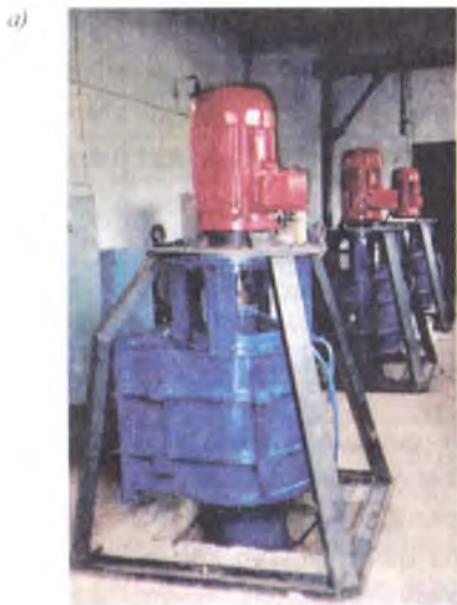
39-rasm. 20 ПрД parrakli diagonal turbinalarining ishchi holatidagi ko'rinishi (a) o'rnatilish sxemasi va (b).
