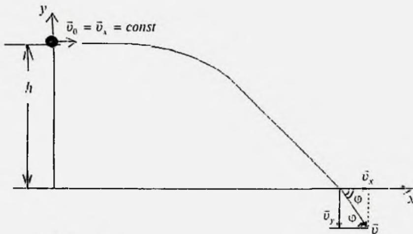
$$\begin{cases} h = \frac{gt^2}{2} \\ v_x = v_0, v_y = gt; \quad v = \sqrt{v_x^2 + v_y^2} = \sqrt{v_0^2 + (gt)^2} \\ \operatorname{tg} \phi = \frac{v_y}{v_x} = \frac{gt}{v_0} \end{cases}$$
