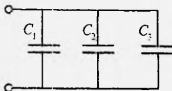
$$C_b = C_1 + C_2 + C_3 = 3 \text{ m}\mu\text{F} ;$$
