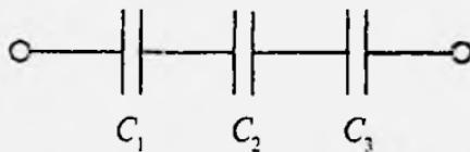
$$\frac{1}{C_b} = \frac{1}{C_1} + \frac{1}{C_2} + \frac{1}{C_3} = 3 \text{ m}\mu\text{F} ,$$
