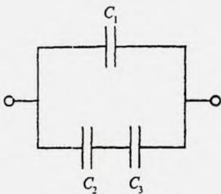
$$C_{23} = C_2 + C_3 = 2 \text{ m}\mu\text{F} ,$$
