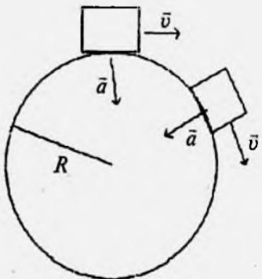
$$a = \frac{v^2}{R} = \frac{15^2 \text{ m}^2/\text{s}^2}{750 \text{ m}} = 0,3 \text{ m/s}^2.$$
