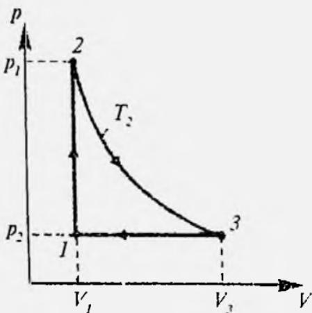
$$\Delta U_{12} = \frac{i}{2} v R (T_2 - T_1), \quad p_1 V_1 = v R T_1,$$
