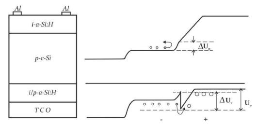
Thus, a three-layer solar cell includes barriers that impede current carriers and create resistance. In the same structure, the main role is played by the heterojunction between the i / p-c-Si and p-a-Si: H layers, because it itself creates a great obstacle for electrons. But for holes, the height of the potential barrier is small. Therefore, holes are the main current carriers. Suppose there is a transfer of holes from the p-c-Si layer to p + -a-Si: H, in this case we have
