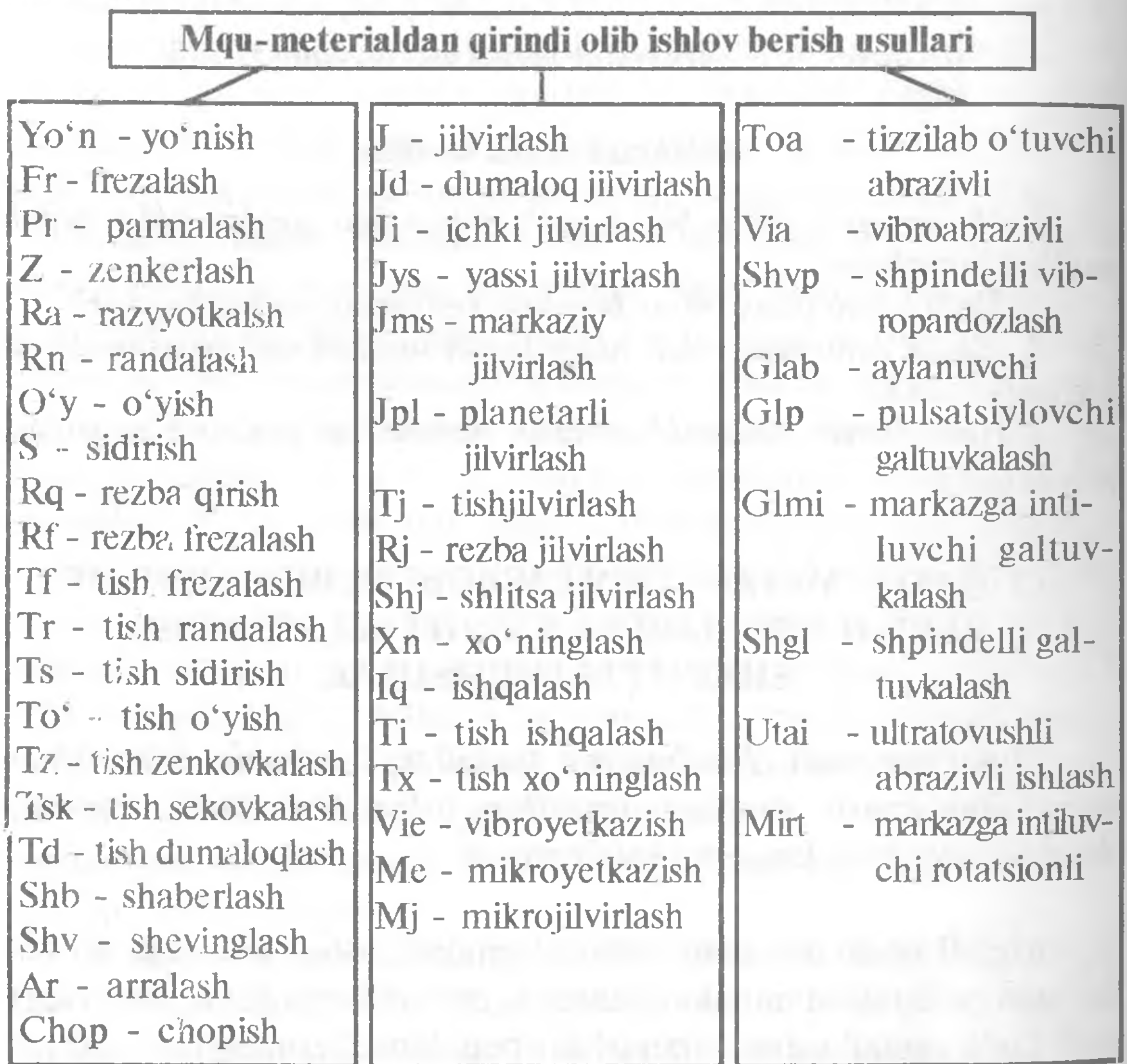
4.4- rasm. Materialdan qirindi olib ishlov berish usullarining tasnifi.
