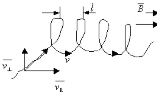
$$F_{\text{Лор}} = \frac{mv_{\perp}^2}{R} \Rightarrow \text{отсюда } R = \frac{mv_{\perp}}{qB} = \frac{mv \sin \alpha}{qB}; \quad T = \frac{2\pi m}{qB}; \quad R = \frac{mv \sin \alpha}{qB}$$
