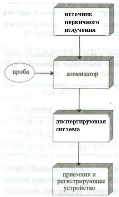
Rice. 1.2.1. Main components of an atomic absorption spectrometer.
