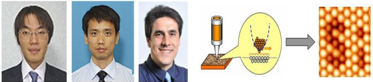
Figure 9. Abbreviation "Si" written on tin with individual silicon atoms by Yoshiaki Sugimoto, Masayuki Abe, and Oscar Kustanse using an AFM probe
